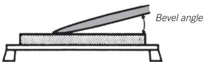
While maintaining the desired angle, use straight movements to grind the blade lengthwise on the stone, and be sure to use the stone's entire surface. Use your right hand to hold the knife's handle and rest your right index finger on the blade. The fingertips of your left hand should be spread close to the cutting edge and used to exert pressure.
