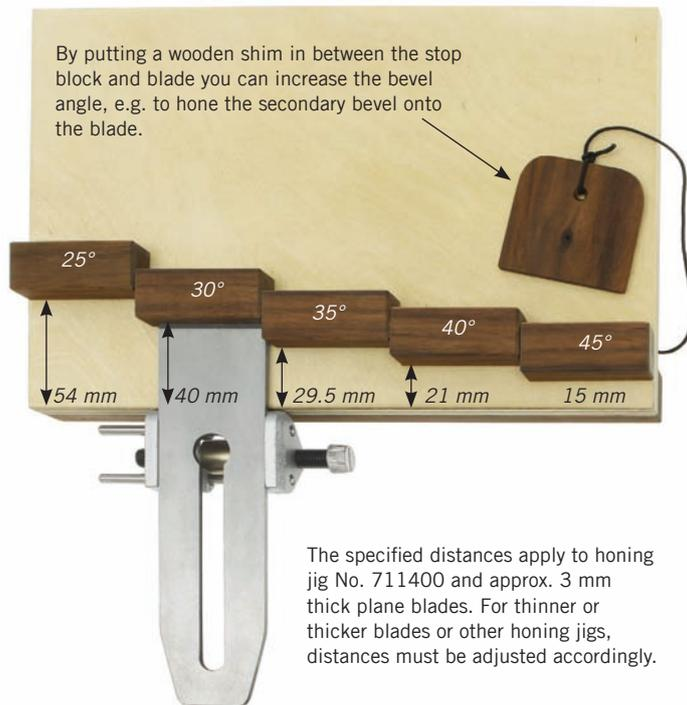
The specified distances apply to honing jig No. 711400 and approx. 3 mm thick plane blades. For thinner or thicker blades or other honing jigs, distances must be adjusted accordingly.
