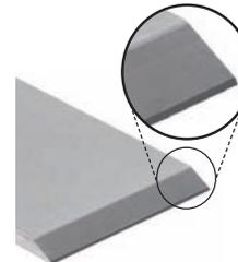
Once you have adjusted the sharpening angle to the required final bevel angle (30°, 35°, 40°, 45°), you hone on a secondary bevel on a finer stone (e.g. 1000 grit). This requires only a few passes across the stone. The result is an ultra-thin secondary bevel that needs to be polished on a polishing stone e.g. 6000 grit.
