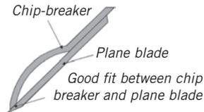
When sharpening thick (Japanese) blades that have a large contact surface area, maintaining a constant angle is easier than with thin blades. One way to check how evenly pressure is being applied is to look at the tracks on the sharpening stone. A honing guide is very useful for helping maintain an exact bevel angle (e.g. No. 707168).
