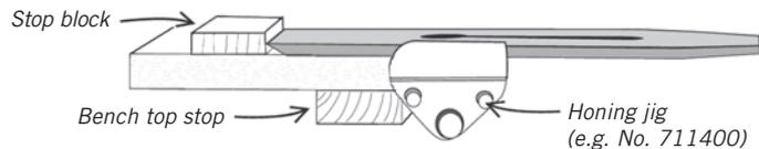
By putting a wooden shim in between the stop block and blade you can increase the bevel angle, e.g. to hone the secondary bevel onto the blade.
