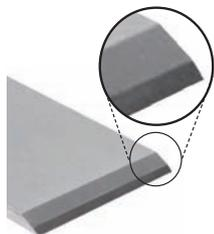
With time, the secondary bevel will become wider and wider, i.e. the surface to polish becomes larger. To speed this up, from time to time you should regrind the primary bevel on the coarsest stone you have to such an extent that the resharpening goes quickly. Alternatively you can use a honing guide and self-adhesive abrasive paper (e.g. No. 707574-707577) [1] stuck on a granite stone plate (No. 711294) [2].
