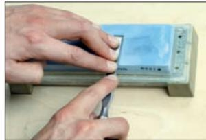
Japanese blades can be trued on diamond blocks (No. 705382) or using a steel lapping plate (No. 713600) and silicon carbide powder (No. 713603 or No. 713604).
