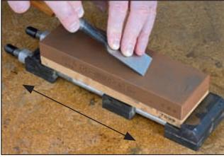
To a large degree, tools are sharpened in the same manner as knives. First, the bevel is ground using a 1000 grit stone. The bevel is placed on the stone diagonally and ground using straight movements while the angle is kept as constant as possible. Rocking and tilting movements should be avoided. In order to work efficiently and to wear the sharpening stone evenly, the entire surface of the stone should be used.
