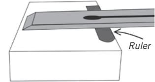
Additionally, you hone a micro-bevel onto the blade. This means that a smoothing plane with a 25° bevel, for example, gets a second bevel (e.g. bevel angle 30°) that is a few degrees less acute.
