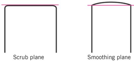
Sharpening guides with barrel-shaped rollers (e.g. No. 703839) 1 allow for honing slight curves into plane blade edges whilst still maintaining an accurate and consistent bevel angle.
